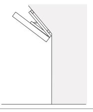
■ Do not install the Wall Mounting Unit on a non-vertical wall.
